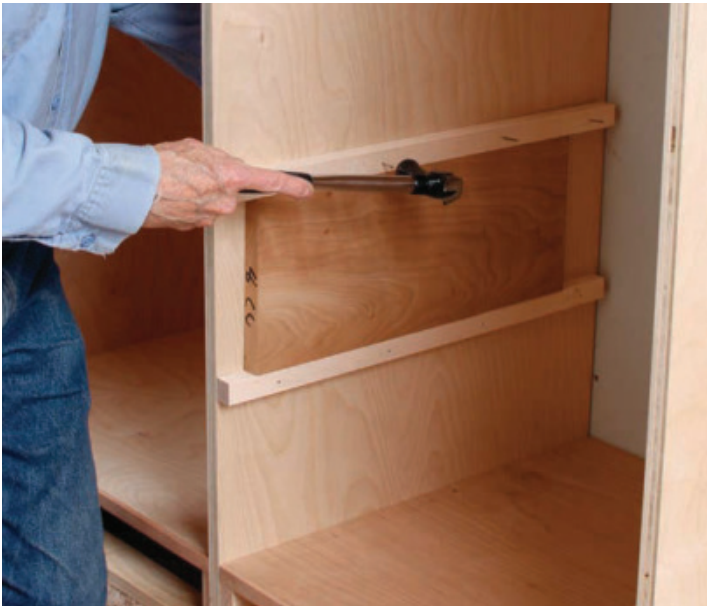
Spacer keeps them aligned. Rest the drawer runners on a simple spacing template as you nail them in place.
