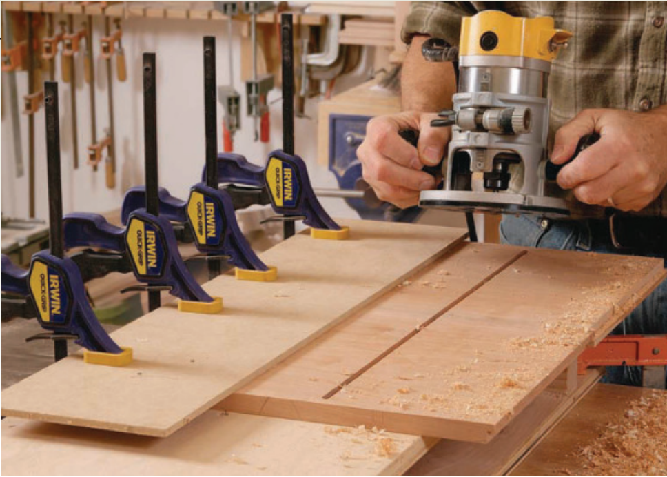
Stopped dados for the vertical divider. Clamp both shelves together with the back edges adjacent. Rout the dados using a straightedge to guide the router base. Stop short of the ends and square up the dados with a chisel.
