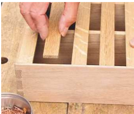
28 Thickness slats to 24 x 5mm and saw to length. These can be pinned or screwed into the rebates
