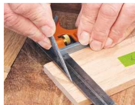
6 Saw sides and ends 2mm over-length for trimming joints later. Scribe shoulder lines for dovetails with a marking knife
