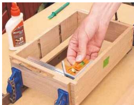
20 Clean up inner surfaces and check for fit. Glue and cramp up the tray, checking for square
