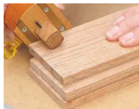
9 Set a gauge to 5mm and mark a rebate for the bottom slats. Pencil in waste to be removed between the tails
