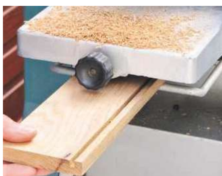
2 Inspect all surfaces closely for defects and cut off damaged ends. Thickness the clean timber to 10mm
