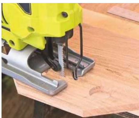
25 Remove remaining waste between holes with a jigsaw. Use this for sawing the tapered edges of the handle
