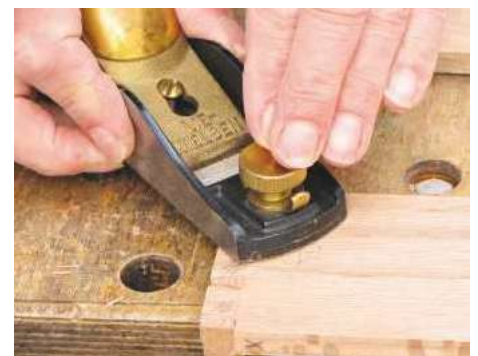
21 Once the glue has dried, trim protruding dovetails flush with a finely-set block plane
