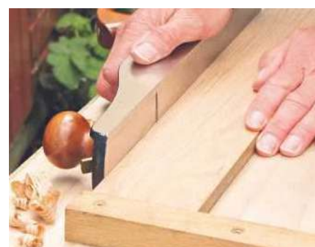
3 True up the face edge of side and end pieces with a bench plane and shooting board. Check with a straightedge
