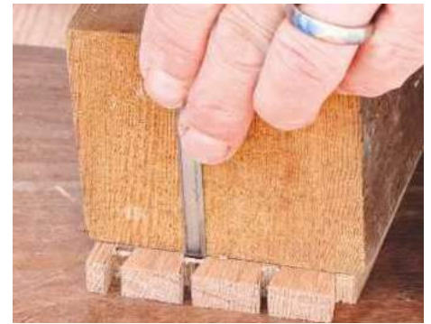
12 Cramp the square timber block along the shoulder line to keep the chisel upright when paring back between tails
