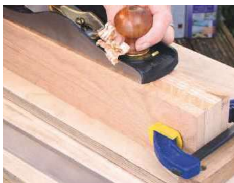
4 Trim ends square on a shooting board. Cramp pieces together, face edge down, and plane to width
