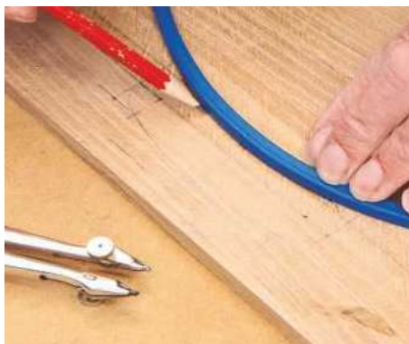
23 Draw the handle cutout with a flexible curve or arched steel rule. Allow enough width for the sanding drum
