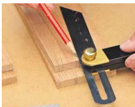
8 Mark out tails with a sliding bevel set at an 1:8 angle (for hardwood). Alternatively, use a dovetail marker gauge
