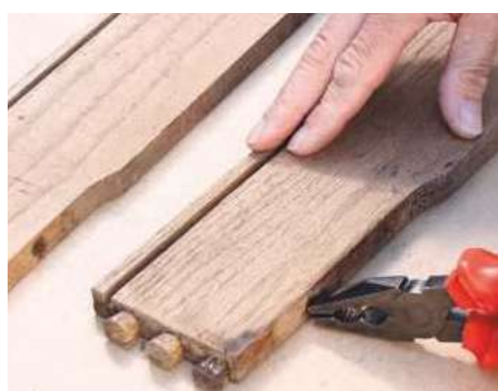
1 When recycling timber always remove old screws or nails first. If rusted, plan saw cuts to avoid defects
