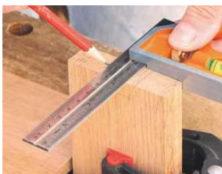
7 Space dovetails to allow for a 5mm rebate at the lower edge. Cramp boards together and square lines across
