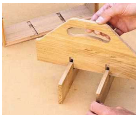
27 The handle and dividers are slotted together. Mark out halving joints and carefully cut away the waste
