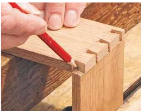
13 Cramp the pin board in a vice and lay the tail piece across horizontally. Carefully mark out pins from the cut tails
