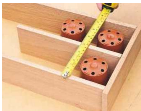
5 Mark each tray component for width and cramp together. Place on a flat surface and plane to width
