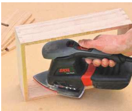
29 Rout a small decorative chamfer along the edges of the tray and dividers. Sand with 180 grit abrasive
