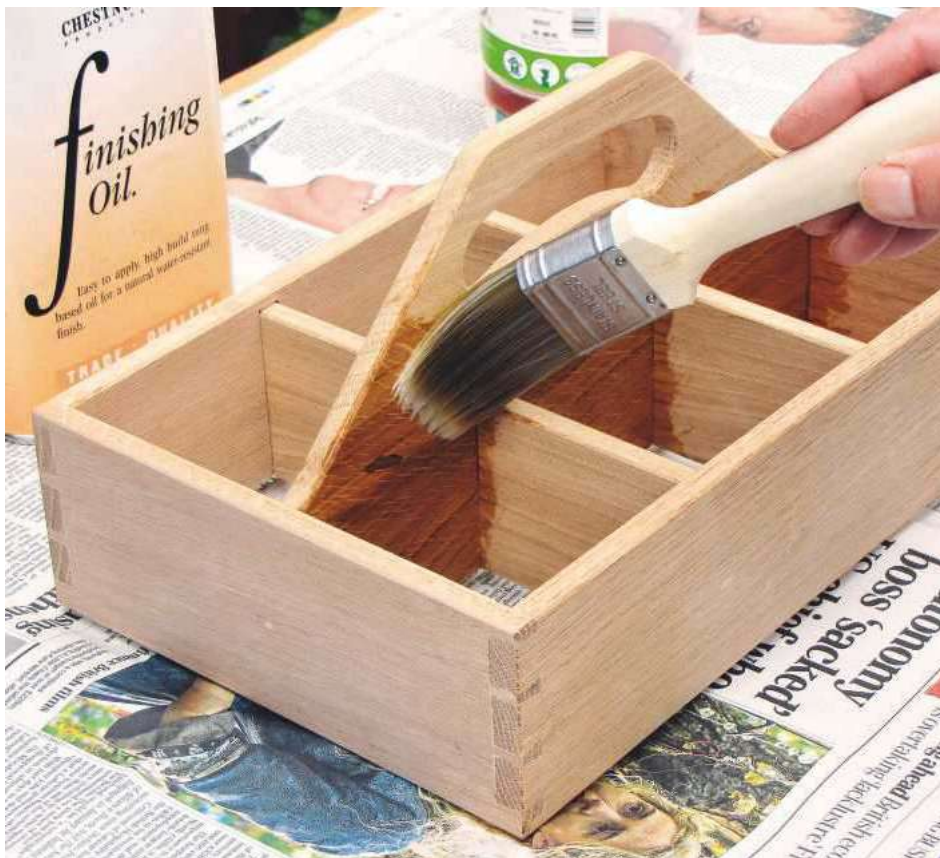
30 Brush on two coats of finishing oil, wiping off after a few minutes. Alternatively, add wax if intended for indoor use
