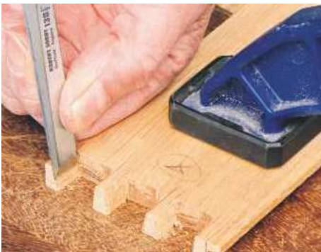
16 Holding the chisel at the correct angle, trim sides of the pins (sockets) as necessary. Check joints fit, and adjust
