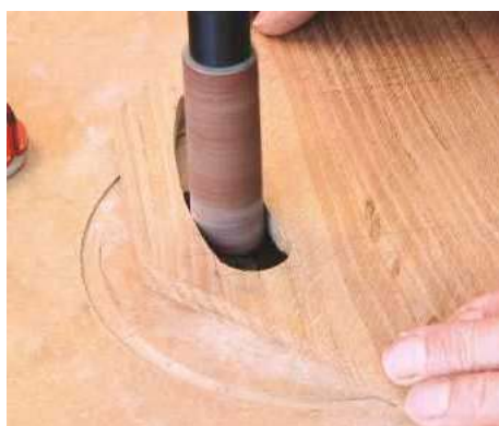
26 Clean up the cutout with a 25mm sanding drum or rasp and file. Smooth edges with abrasives
