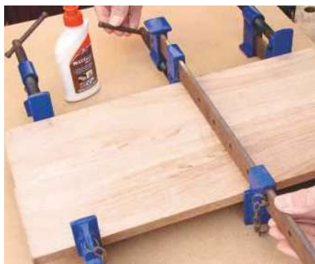
22 If required, glue boards together to achieve sufficient width for the carrying handle. Thickness when dry
