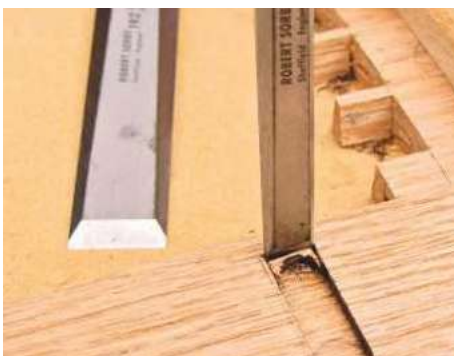
19 Housings are stopped 5mm below the top edges. Square rounded ends neatly with a chisel
