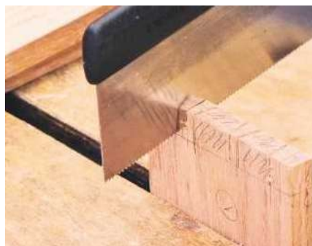
14 Pencil in waste between the pins. Saw down sides of the pins to form the sockets, keeping the blade level
